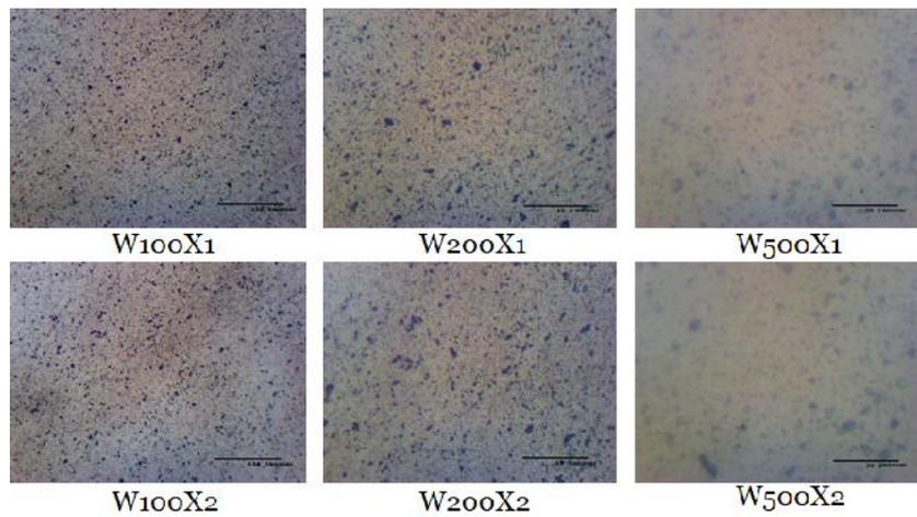
**Figure 8: 6061 FSW S=1000 F = 80 Weld Portion**
