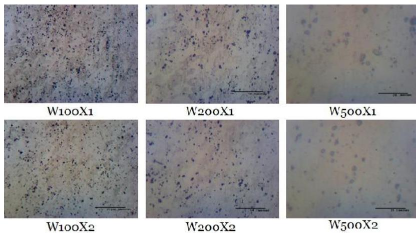
**Figure 9: 6061 FSW S=1000 F = 100 Weld Portion.**
