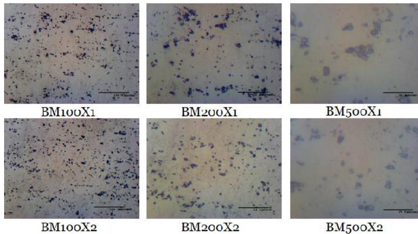
**Figure 6: 6061 FSW S=1000 F = 100 Base Metal**
