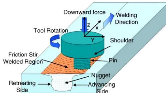
**Figure 1: Diagrammatic Representation of the Friction Stir Welding Process [6].**
