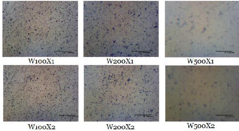
**Figure 7: 6061 FSW Weld Portion S=1000 F = 63.**
